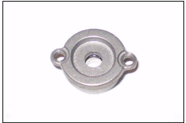
Figure 50. Camshaft Faceplate, Modified for the Shaft Extension
