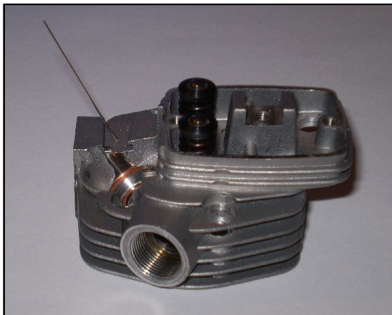
Figure 42 & 43. Pictures of Cylinder Head with Hypodermic Needle
