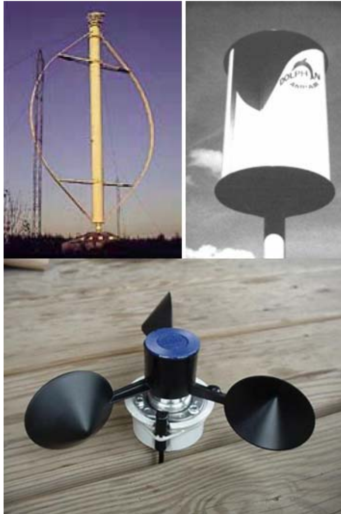
Figure 5.2.2: Pictures of Different Types of Vertical Axis Wind Turbines: Airfoil (Top Left), Savonius Rotor (Top Right), and Cup (Bottom).
