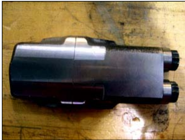
Figure 17: One of two connecting rod samples ready for testing.
