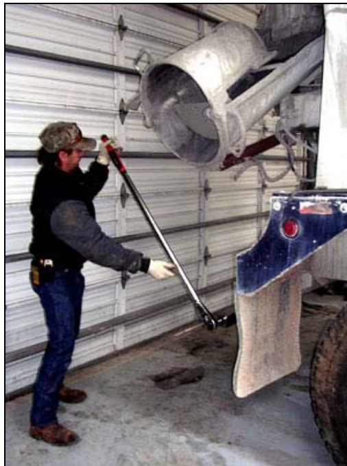
Figure 22: Florida rock applying the 330ft-lb torque to the main bearing cap bolt.
