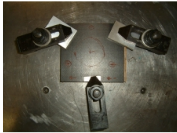
Figure 14.1 – Fabricating Bulkheads on CNC
