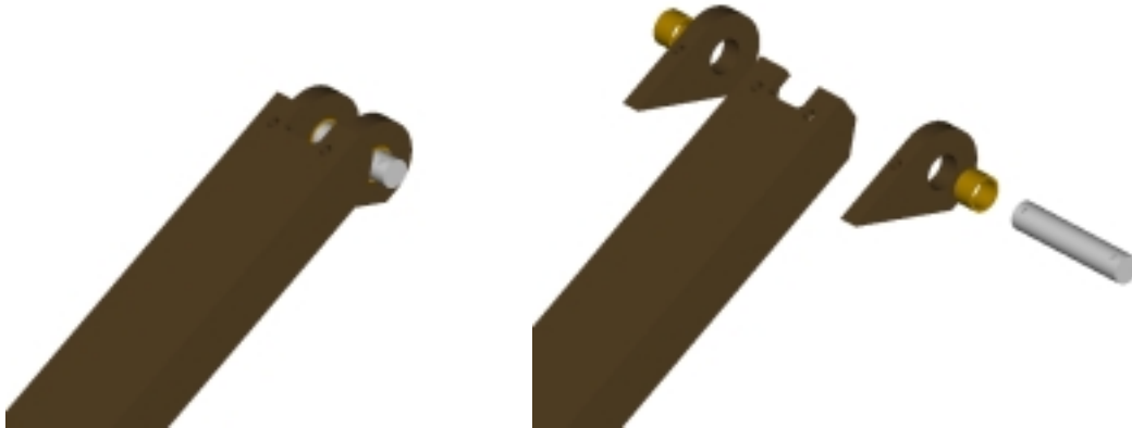
Figure 8.5 – Lifting Arm End Clevis Joint
