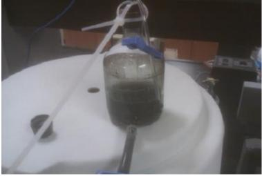
Figure 1 – 50:50 leachate:sludge under anaerobic conditions.
