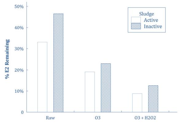
Figure 1 – Degradation of E2 in Leon County leachate under anaerobic conditions (batch) after pre-treatment with ozone or 'peroxone' ( $H_2O_2 + O_3$ ). Incubation: 24 hrs.
