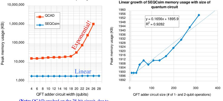
(Note: QCAD crashed on the 28-bit circuit, due to insufficient memory available on the test PC.)
