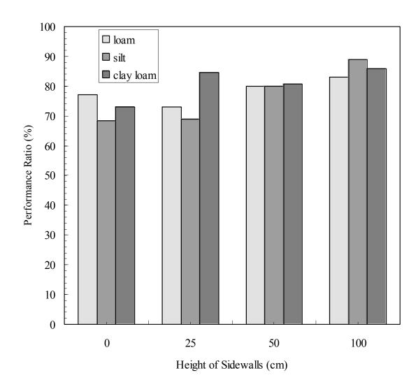
Fig. 4.8 Performance Ratio of Large Lysimeters With Sidewalls on Slopes 1:4 After Two Years Simulations.
