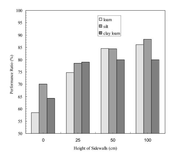
Fig 4.5 The Performance Ratio of Medium Lysimeters With Sidewalls After Two Years Simulation.
