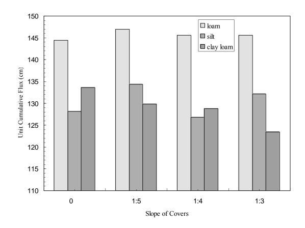
Fig 4.1 BaseLine Unit Cumulative Flux of Full Scale Covers After Two Years Simulations.
