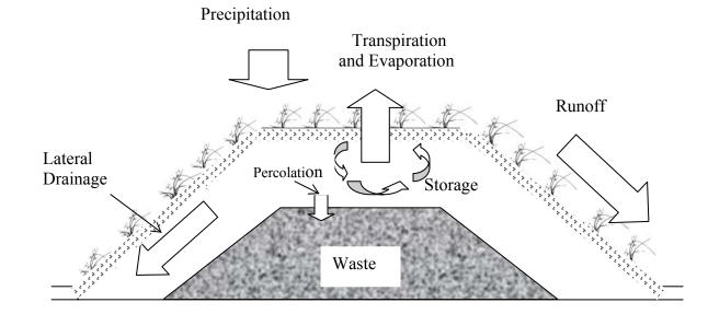
Fig. 2.2 Profile of Evapotranspiration Cover.
