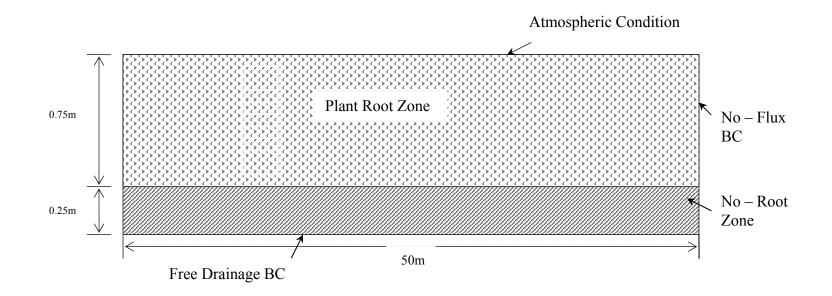
Fig. 3.3 Sketch of Simulation With Full Scale Cover.
