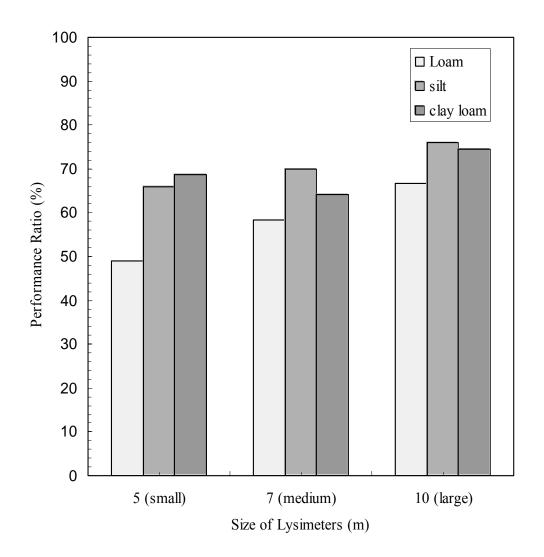
Fig. 4.6 The Performance Ratio of Large Lysimeters With Sidewalls After Two Years Simulation.
