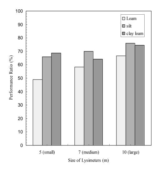
Fig.4.2 Performance Ratio of Lysimeters Without Sidewall After Two Years Simulation.
